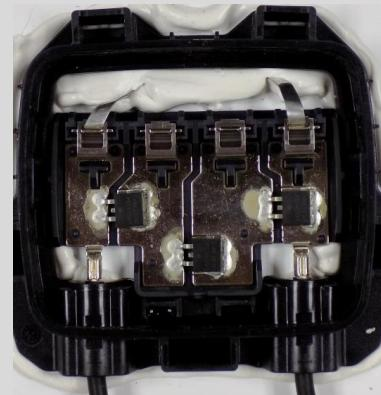
**Fig 4: detail view of open Junction Box**
